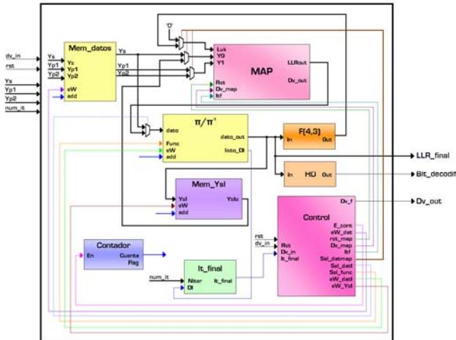
Figure 7. Block diagram of the implementation of turbo decoder, N=1024.
