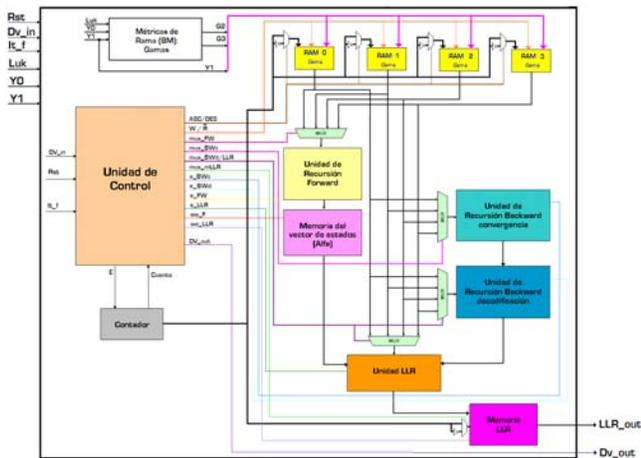
Figure 8. Block diagram of the implementation of decoder SISO, N=1024.
