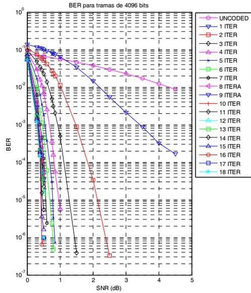
Figure 6. Results of BER of the simulation for N = 4096 3GPP [4].
