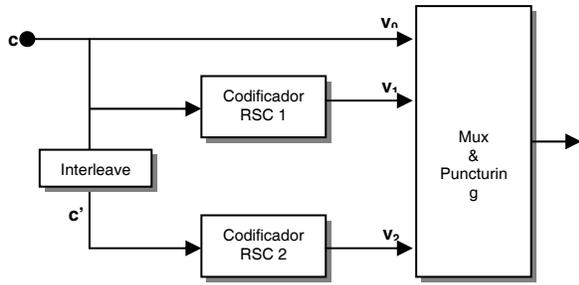
Figure 1. General structure of a turbo encoder.
