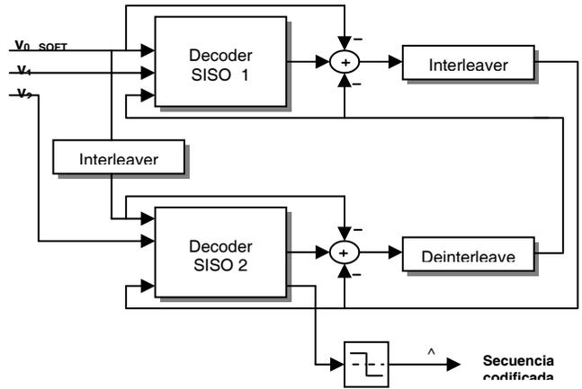
Figure 3. General structure of a turbo decoder
